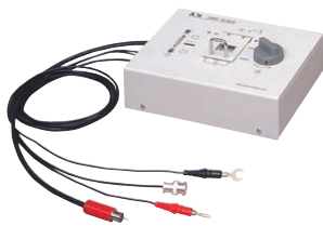
External Dimensions: Approx. 200 (W) x 52 (H) x 150 (D) mm, Lead Length: Approx. 85 cm, connects with special Hioki plug.
