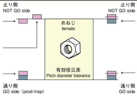
止り側 NOT GO side      止り側 NOT GO side<br>めねじ female<br>有効径公差 Pitch diameter tolerance<br>通り側 GO side (prod/insp)      通り側 GO side                 | NP                                                                 | 4H         | 通り<br>GO                                                                                    | 止り<br>NOT GO                                               |
